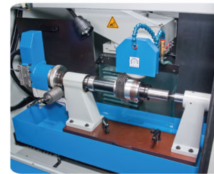
G320B Knife Back Grinding (Finger jointer knife)
