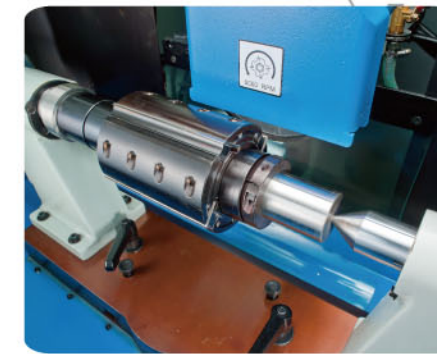
G320B Knife Edge Grinding (Movable straight knife)
