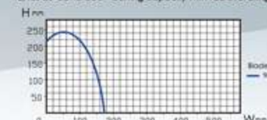
T5/T5S 30" Sawblade - Cutting capacity with table rotating 90°
