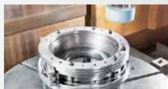
煞車環端面+內外徑研磨
