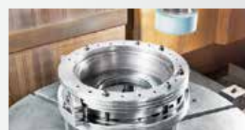
煞車環端面+內外徑研磨
