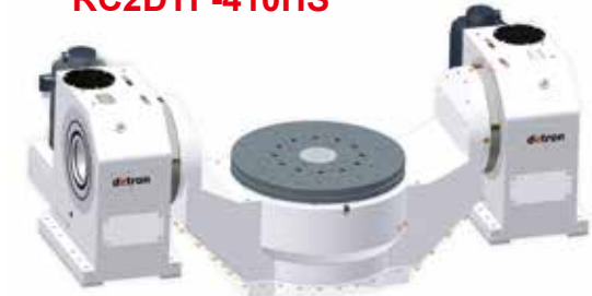
Rotary Axis - DDM (1200rpm) Tilting Axis - Tandem drive by spur gear and worm gear
