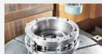
Finishing grinding for brake drum face+ID+OD
