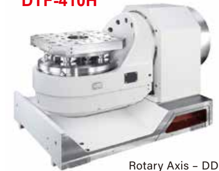
Rotary Axis - DDM (1200rpm) Tilting Axis - Tandem drive by spur gear and worm gear
