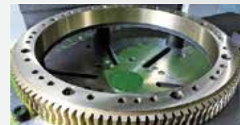
Finishing grinding for gear face
