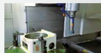
Finishing grinding for casting ID
